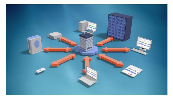
Several wayside eRDM systems can be integrated into a redundant high availability diagnostic server solution. The server collects, stores, processes, and analyses the measurement results and sends the alarm and warning signals to client computers installed in operational stations.
