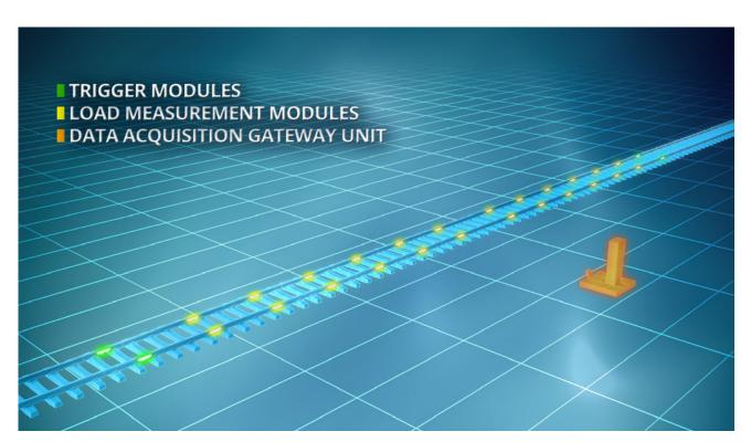
The measured high resolution load response signals are sent to the data acquisition and communication module located near the measurement section. The module has a battery equipped power supply and a wide area network connection (GSM, GPRS, HSPA, DSL etc.) The system analyses the measured axle-time profile using the offline vehicle database. The data acquisition module can be accessed by local Ethernet or Wi-Fi terminal by service maintenance personnel.
